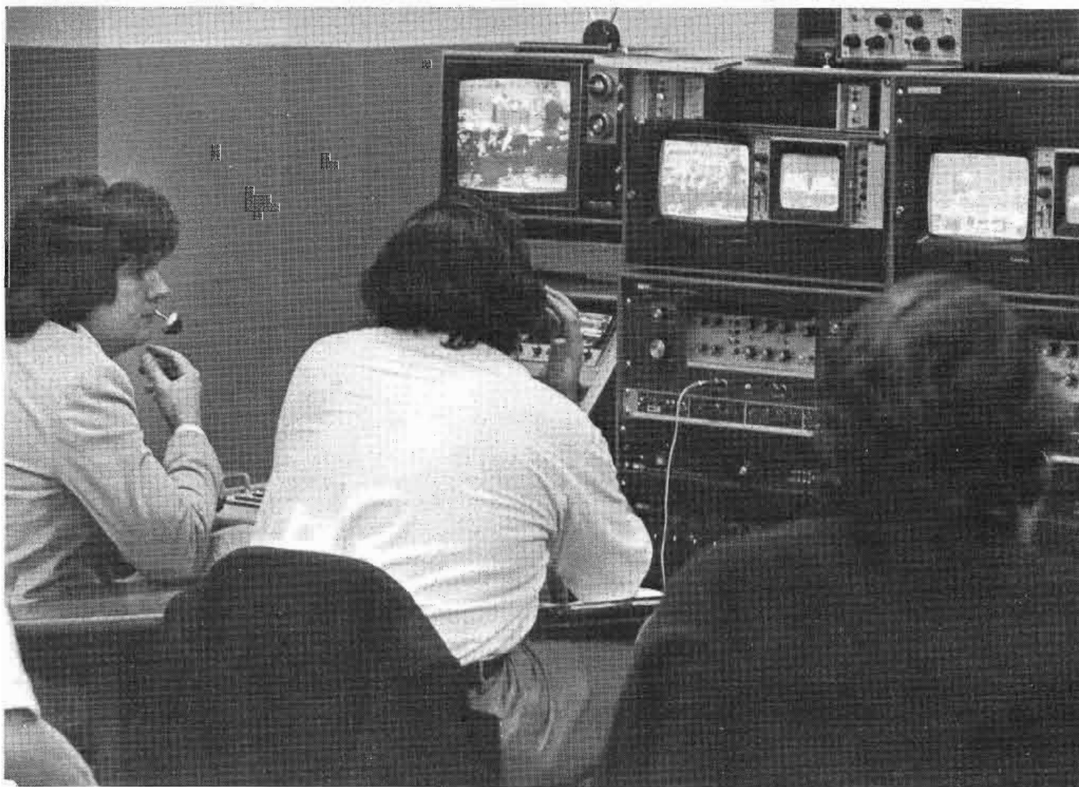
A complete run-through is important before a production to completely check headset communication, mike feeds and camera viewpoints. Set up here was on location at high school gymnasium.
